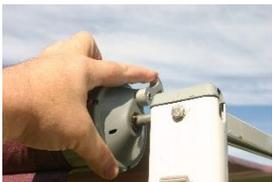
4. Engage end brake lock toggle to roll up position allowing the cloth to tighten against the awning rafters, adjust rafters to tighten cloth if necessary.
