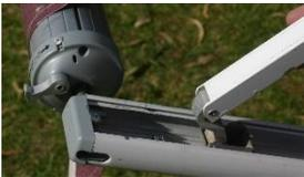
2. Slide awning rafters up the main awning support (leg) and lock into position and tighten rafter black adjustment knob to hold in position.
