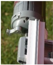
1. Pull down awning and align the awning groove in line with the bolt in the top of the awning leg
